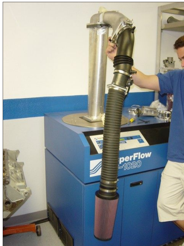
The entire KB Cool Air Kit with production inlet manifold is flow tested.
