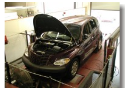
We monitor and data log many vehicles functions during a test. We typically dyno test in 3rd gear. In this test, we recorded HP from 0-115 mph in all 3 gears.
